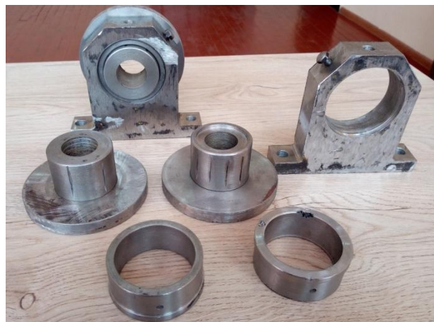
Figure 3. Fifth class rotational kinematic pair components
