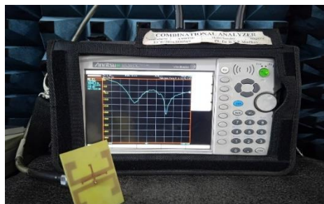
Fig. 8. c) Antenna connected to the Spectrum Analyzer
