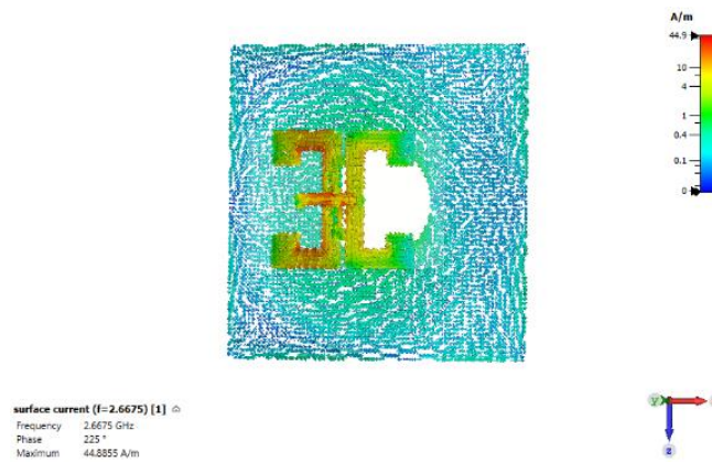
Fig. 3. Current distribution of the patch antenna c) with circular aperture in reflector
