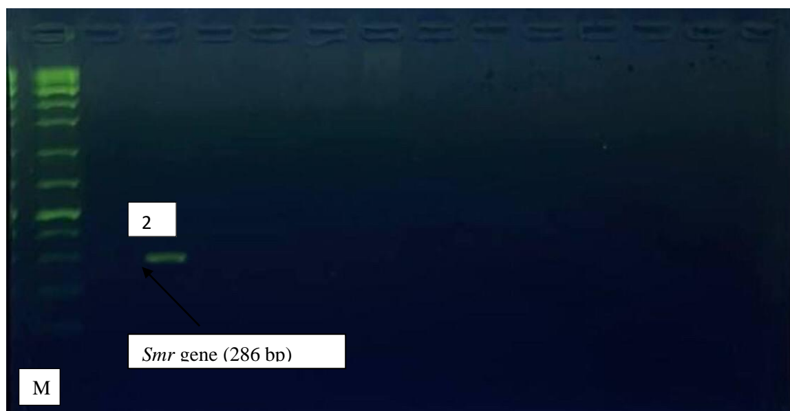
Figure (7) PCR product the band 286 bp. The product was electrophoresis on 1.5% agarose at 5 volt/cm 2 . 1x TBE buffer for 1:30 hours. M: DNA ladder (1000 PLUS).
