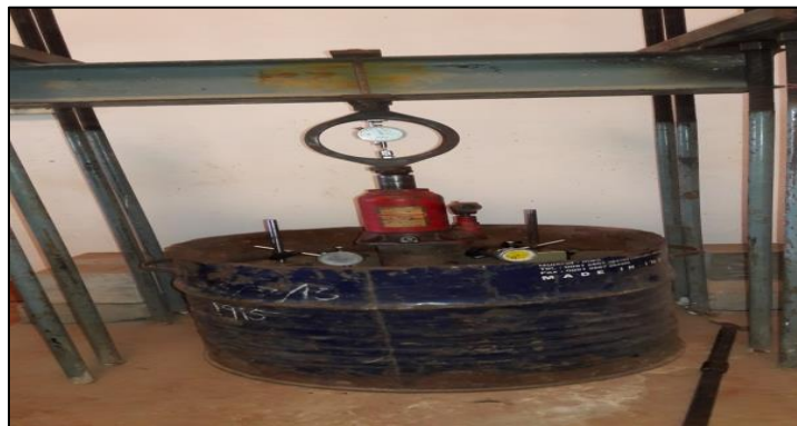
Fig 4.1 Experimental Setup for Cyclic Plate Load Test
